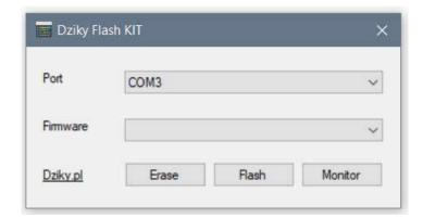
Firmware: Pick up from firmware list software that You want to upload to You ESP Chip.
